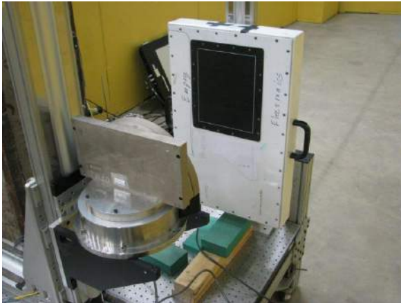
Image Panel, CT stage and uranium plates + test assembly in a WNR high-energy neutron flight path (15R).
