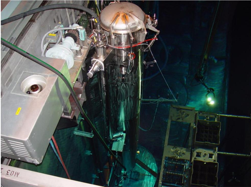
Spent fuel assembly calorimeter at the SKB CLAB facility Sweden
