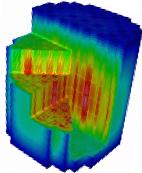
Watts Bar reactor modeling performed under the CASL project.
