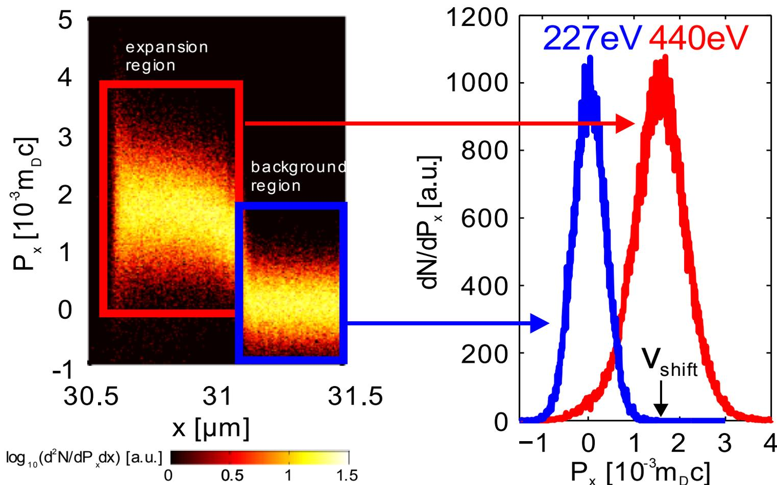
Internal expansion region: ion beam kinetic energy transferred to ion thermal temperature → enhanced ion heating
