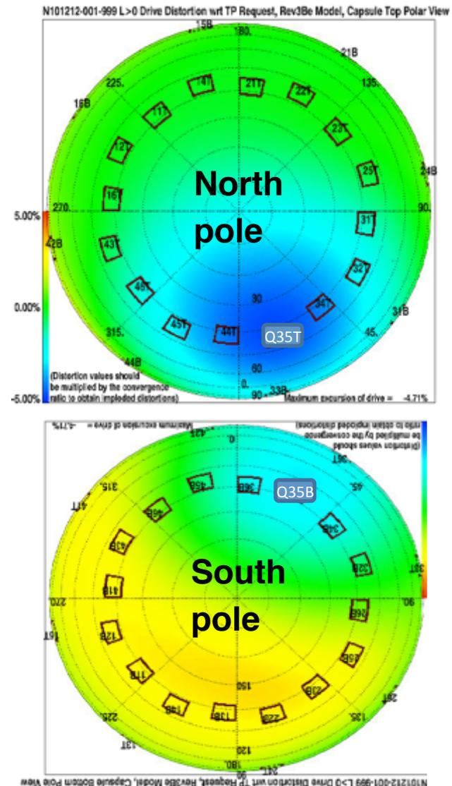
**Core fuel velocity correlates with drive distortion, Doppler-shifting neutron spectrum, increasing activation along velocity axis.**
